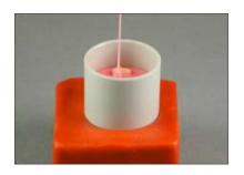
A duplicate of the master model or the master die is fabricated using duplicating material and refractory die material. A thin coat of vaseline is applied to the duplicating base and the duplicating ring; then the master die can be fixed on the duplicating base. A thin stream of duplicating material is poured into the mold to avoid the formation of bubbles. The processing time is approx. 6 min.
