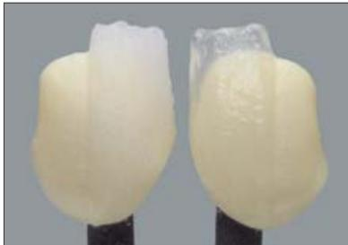
A slight luster of the ceramic surface is an evidence for correct firing. If the ceramic, however, appears to be milky and non-homogeneous, the firing temperature is too low. Approach the correct firing temperature in steps of 5–10°C.
