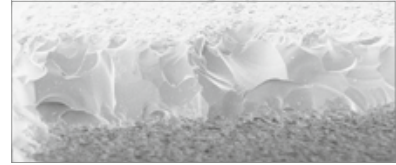
VITA ENAMIC, 30° wedge, lateral view (left photo); VITA ENAMIC, 30° wedge, top view, 200 x magnification (photo in the middle); IPS e.max CAD, 30° wedge, top view, 200 x magnification, (right photo): source: VITA R&D
