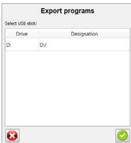
Fig. 13: Selecting the drive (= USB flash drive)
