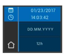
Pressing the date field in Settings allows the user to switch the type of display between DD.MM.YYYY and YYYY.MM.DD, as well as between the 12 and 24 hour display.
