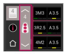
If the measurement memory already contains measurements, it is possible to navigate within the recorded data by touching the Arrow symbol.
