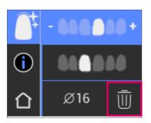
Measured values can be individually deleted and the measurement repeated.
