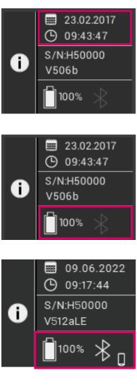
When you tap "Date and Time" in the upper section, you are taken directly to the settings, where you can make changes to the date and time. The serial number and the software version are displayed in the middle area.
