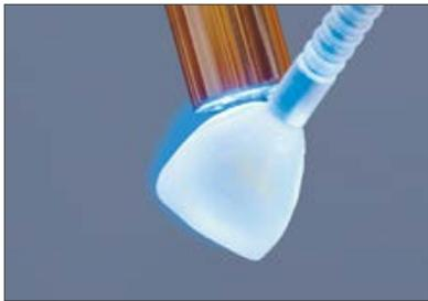
Cure the die material using a light-curing unit or a hand-held curing light (see table).
