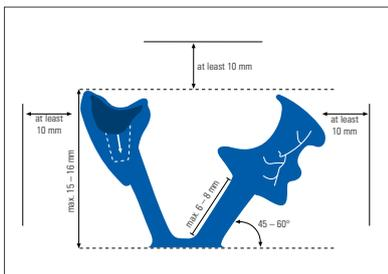
**Correct spruing for the substructure-free staining and layering technique**
