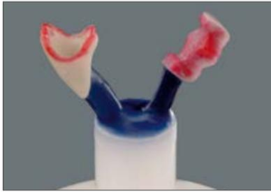
Attachment points between the press sprue, press object and the ring base must be rounded. Sharp edges and narrow points must be avoided. The sprues must not taper towards the wax-up (shaped like a trumpet).
