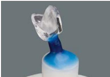
Sprued anterior mould made from VITA CAD-Waxx.
