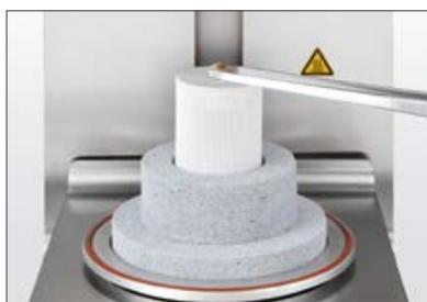
Inserting the VITA PM 9 press pellet
