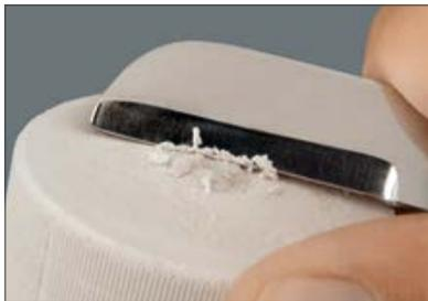
The level gauge determines the height of the investment material mould and the straight position in the press furnace. Any defect on the base must be smoothed or carefully removed with a plaster knife.
