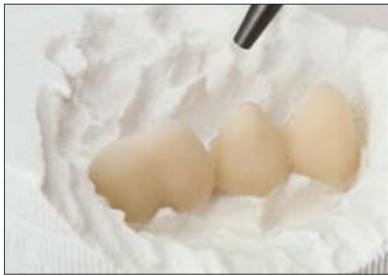
Sandblast with glass beads with a grain size of 50 µm at a pressure of 4 bar.
