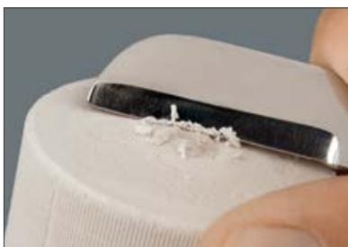
The level gauge determines the height of the investment material mould and the straight position in the press furnace. Any defect on the base must be smoothed or carefully removed with a plaster knife to ensure vertical position of the mould in the press furnace and to eliminate problems during pressing.
