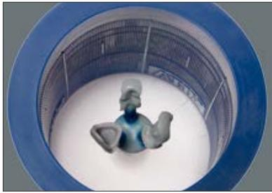
If several restorations are to be pressed, they must be aligned symmetrically in the center of the ring.
