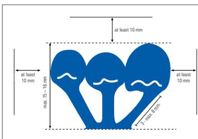
Press object and press sprue should form a single line to allow unobstructed pressing of the ceramic.
