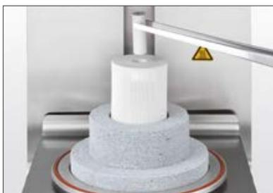
Place the disposable press plunger with the black marking facing upward. The front, which features slightly rounded edges, must face downward.
