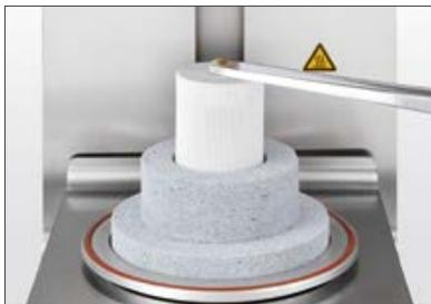
Inserting the VITA PM 9 press pellet.
