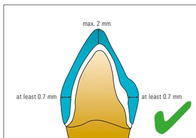
**Minimum wall thicknesses in mm and minimum connector areas in mm<sup>2</sup> for zirconia substructures**
