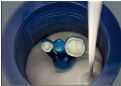
Pour a thin stream of investment material into the investment ring up to the marking, and avoid the formation of bubbles.
