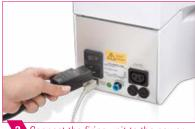
Connect the firing unit to the power supply.
