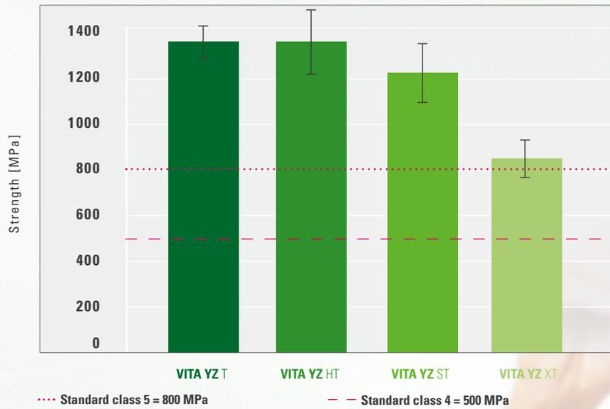
Source: Internal study, VITA R&D, 3-point flexural strength of the different VITA YZ materials according to DIN EN ISO 6872:2015 + Amd.1:2018, (Gödiker, 08/2022, [2] see back of brochure)
