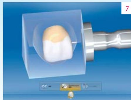
**Fig. 7** The nesting of the crown restoration directly before milling.
