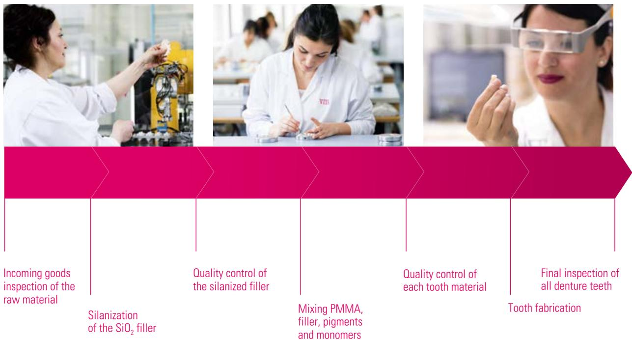
Figure 9: Manufacturing process of VITA denture teeth; source VITA R&D
