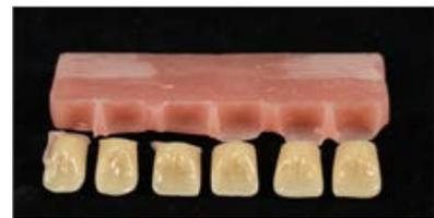
Figure 15 b: Fracture pattern; tooth base was not surface-conditioned
