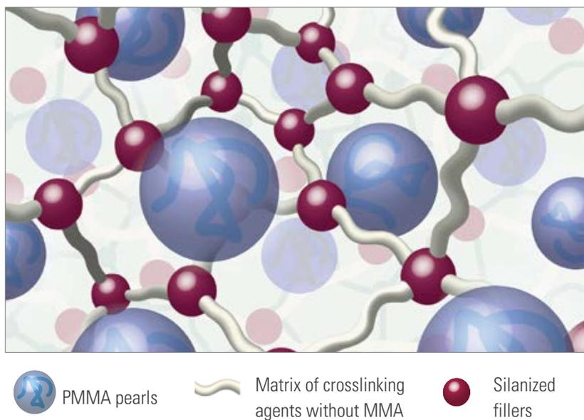
Figure 7: Schematic structure of MRP composite; source VITA R&D
