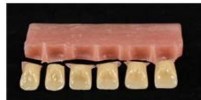
Figure 15 d: Fracture pattern; tooth base was only coated with bonding agent
