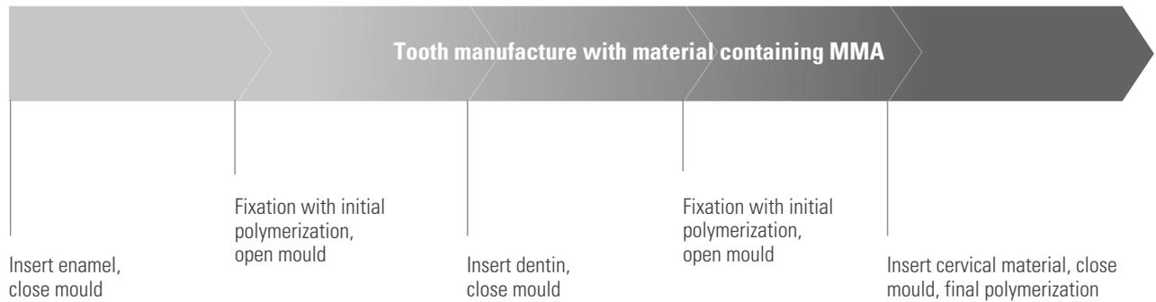
Figure 12: Schematic illustration of manufacturing procedure of (P)MMA denture teeth; source VITA R&D
