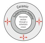
The ideal tangential and radial tensile stress is ensured if the CTE of the ceramic has been optimally matched with the CTE of the substructure material.
