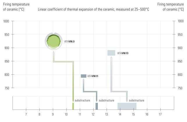
Linear coefficient of thermal expansion of the ceramic, measured at 25–500°C (alloys - measured at 25-600°C)
