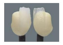
A slight luster of the ceramic surface is an evidence for correct firing. However, if the ceramic appears to be milky and non-homogeneous, the firing temperature is too low. Approach the correct firing temperature in steps of  $5-10^{\circ}$ C.
