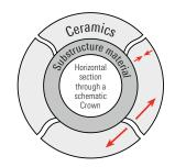
If the CTE of the substructure material is considerably lower than the CTE of the veneering ceramic, tangential tensile stress will increase and form radial cracks that run to the outside. This may result in late cracks.
