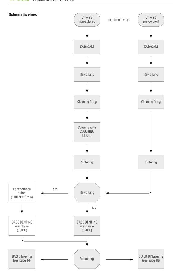
The restorations should be cleaned in distilled water and grinding dust should be removed prior to the application. Cleaning firing should be performed on a fibrous pad in a ceramic furnace (e.g., VITA VACUMAT) to remove the cooling and lubricating liquid from the porous structure.
