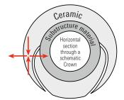
If the CTE of the substructure material is considerably higher than the CTE of the veneering ceramic, tangential compressive stress will increase and form cracks that run almost parallel to the substructure. This may result in chipping.
