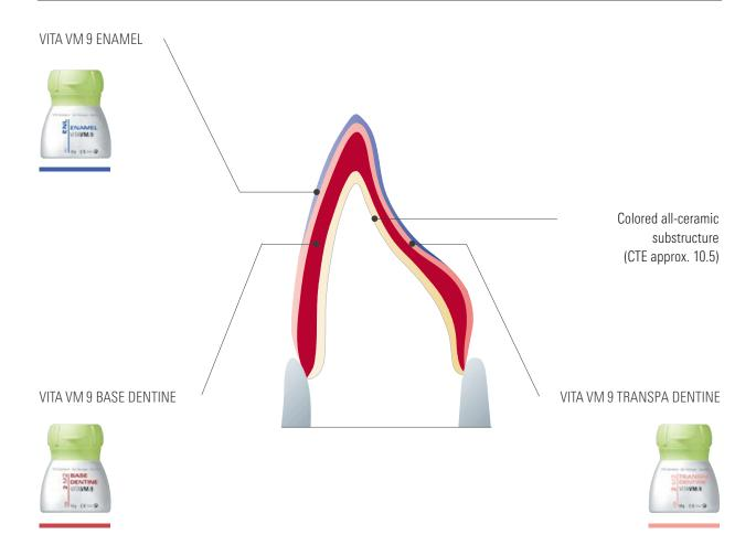
The VITA VM 9 BUILD UP layering includes the application of the three materials BASE DENTINE, TRANSPA DENTINE and ENAMEL.
