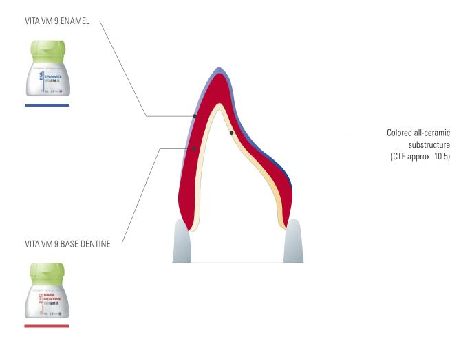
VITA VM 9 BASIC layering consists of the application of the two materials BASE DENTINE and ENAMEL.
