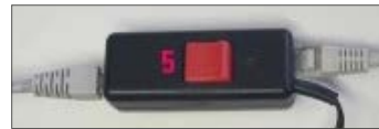
1/5 = on-switch / off-switch only for the vPad, furnace is switched on/off via the main switch
