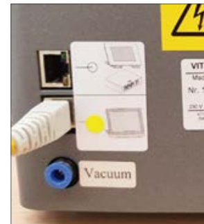
Furnace/connecting cable (yellow point + ring)
