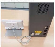
The vPad is connected directly to the furnace
