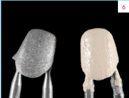
Fig. 6 The CTE buffer VITA NP BOND was applied to the non-precious metal substructure and fabricated with the support of CAD/CAM.
