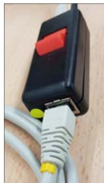
Injector/connecting cable (yellow point + ring)
