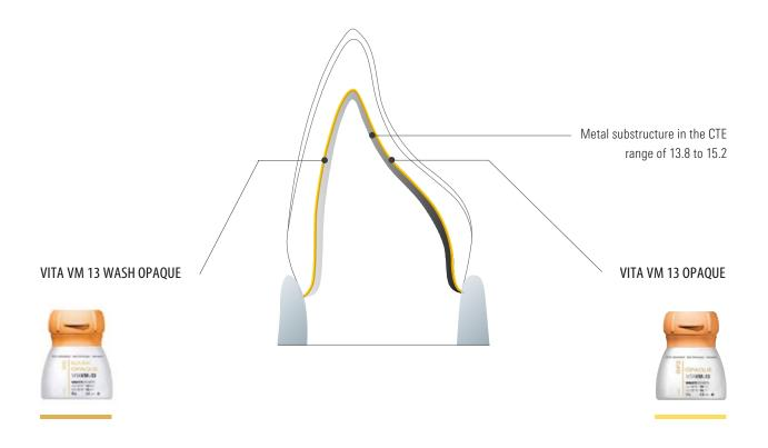
To prepare the VITA VM 13 BASIC and BUILD UP layering, first apply WASH OPAQUE and OPAQUE to the substructure.
