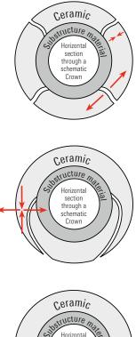
If the CTE of the substructure material is considerably lower than the CTE of the veneering ceramic, tangential tensile stress will increase and form radial cracks that run to the outside. This may result in late cracks.
